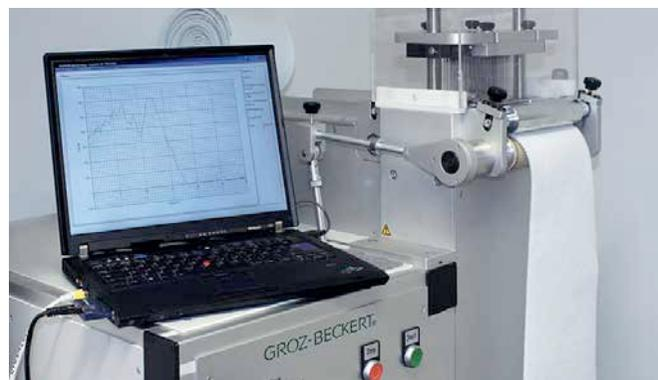
Measurement of penetration force and mechanical work
