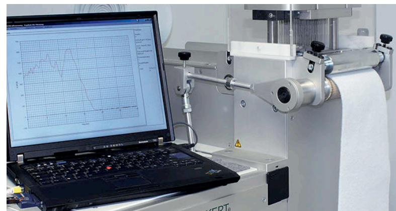
Measurement of penetration force and mechanical work
