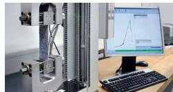
Testing tensile force and elongation
