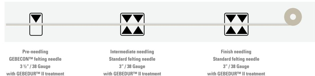
GEBECON™ felting needles used for pre-needling offer the perfect combination of good surface properties in the end product and optimum bending strength. Treating the felting needles with GEBEDUR™ II over the complete needling process guarantees an extended service life and consequently a uniform needling effect for the whole application period.
