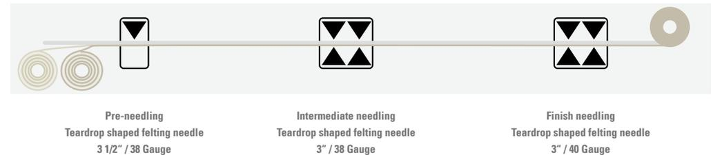
Felting needles with a teardrop shaped working part cross-section and HL barbs over the whole needling effect enable products to be manufactured causing minimal stress to the fibers and low damage to the support fabric.
