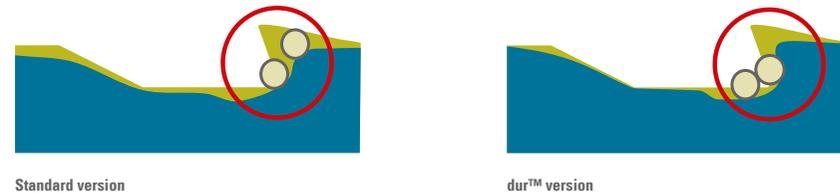
Barbs and forks, produced with the “dur™” technology, maintain their original shape longer compared to the standard version and are able to provide the same efficiency over a longer period of time. As a result, a lower punch density may be utilized resulting in increased productivity.
