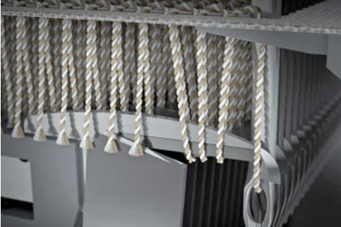
Pick-up of the loop by the looper
