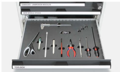
Drawer 3: Storage place for major tools; for other tools the foam can be cut to size
