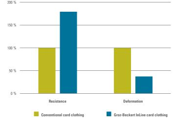
Resistance and deformation of a doffer wire tooth with load
