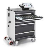
The **needle dispensing trolley** replaces the needle dispensing desk and is used to store new needles and various tools. In addition, it serves as a collection point for used and broken needles.
