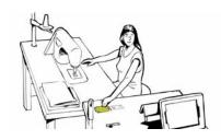
The operator takes the closed box and inserts the new needle into the machine.
