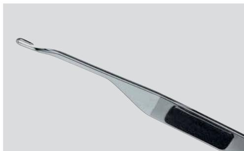
For gauges from E 40, Groz-Beckert has developed and patented a special compound needle with thickened plastic part. The special feature of needle Spec. 51/ 43.36 G 101 is that its lateral thickened plastic part lends the fine needle adequate stability during loop formation.
